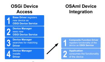
Fig. 1. Sequences in OSGi Device Access and OSAmI Device Integration
